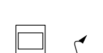
PD-VSENS CASÉTA VACANCY SENSOR 180° COVERAGE 4.35"[110mm] (H) X 1.8"[46mm] (W) X 1.35"[34mm] (D) *DEVICE CAN BE WALL-MOUNTED AND IS BATTERY POWERED (POWER FEED NOT REQUIRED) LOCATION TBD
